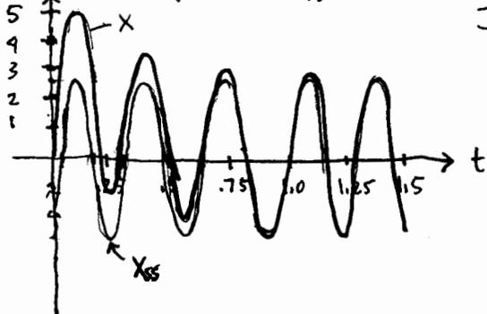
In about 4 or 5 characteristic times  $\tau_1$  (about  $t = 1 \sim 1.25$ ) the transient dies away & you only see the steady state:
