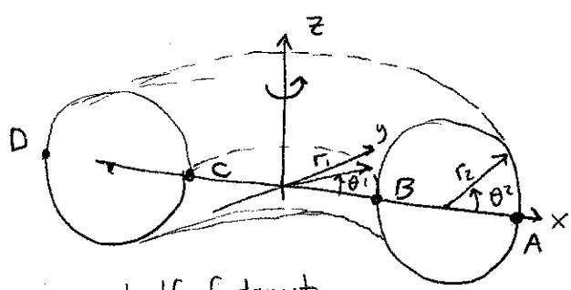
revolve the circle in the  $z$ - $x$  plane centered at  $(r_1 + r_2, 0, 0)$  around the  $z$ -axis. Call this  $T^2$ .
