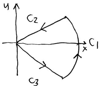
$C_1: x^2 - 2x + y^2 = 0 \rightarrow x = \frac{2 \pm \sqrt{4-4y^2}}{2} = 1 \pm \sqrt{1-y^2} \rightarrow + \text{sign.}$
