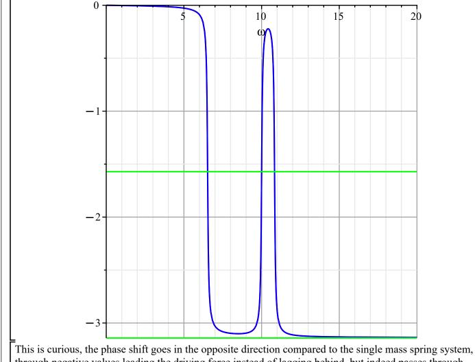
through negative values leading the driving force instead of lagging behind, but indeed passes through negative 90 degrees quickly to 180 degrees passing through the first resonance frequency. It then briefly returns towards zero as it passes through the second resonance and then returns to 180 degrees. I do not understand this. It requires more investigation.
