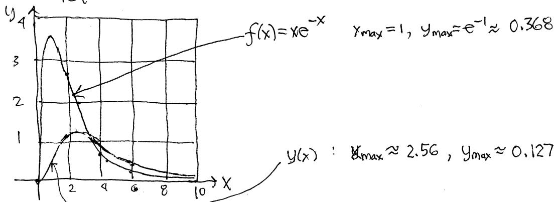
E8P3 5.5.9 method of undetermined coefficients: root overlap case
