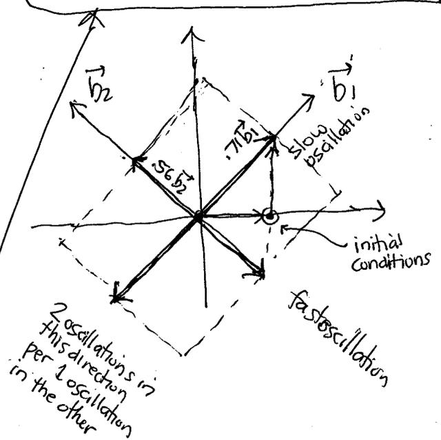
2 oscillations in this direction per 1 oscillation in the other so we have to get a figure 8 like curve
