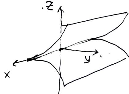
Intersection of any two of these surfaces describes the unparametrized curve
