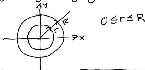
$$V = \frac{P}{4\eta l} (R^2 - r^2) = \underbrace{\frac{PR^2}{4\eta l}}_{V_{max}} \left(1 - \left(\frac{r}{R}\right)^2\right)$$
