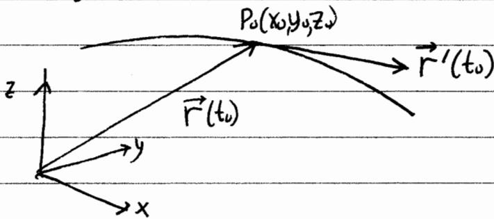
One can think of the tangent space at  $P_0$  as the space of tangent vectors at  $P_0$  to all possible parametrized curves passing through  $P_0$ . This is in fact a useful idea which generalizes to more complicated settings.
