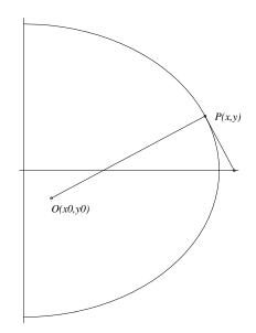
FIGURE 1. The normal line segment from the given point O and the point P together with the tangent line segment from P to a point on the major axis, a configuration whose geometry led Apollonius to the hyperbola whose intersection with the ellipse determines its normal lines.
