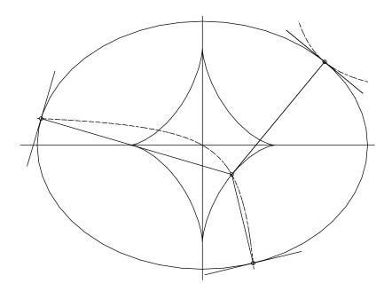
FIGURE 5. As the point approaches the evolute from inside (not at one of its vertices), two of the four normals coallesce as one branch of the hyperbola of Apollonius becomes tangent to the ellipse, in the first quadrant in the configuration shown here.
