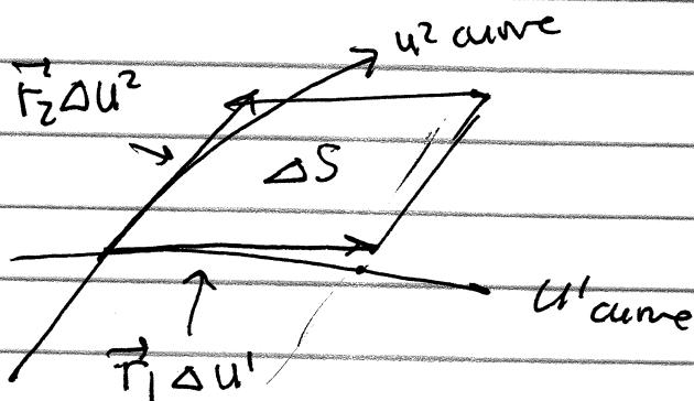
$$\Delta S = |(\vec{r}_1 \Delta u^1) \times (\vec{r}_2 \Delta u^2)| = \underbrace{|\vec{r}_1 \times \vec{r}_2|}_{|\vec{N}|} \Delta u^1 \Delta u^2$$
