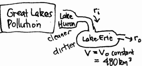
$$r = r_i = r_o = 350 \text{ km}^3/\text{yr} \text{ (no accumulation of water)}$$
