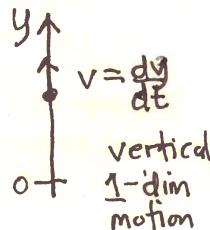
acceleration  $\sim$  gravity down
