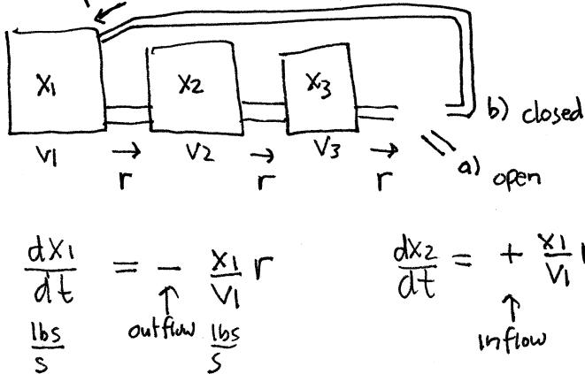
$$\left\{ \begin{array}{l} r = \text{rate of solution flow gal/s} \\ x_i = \text{amount of solute lbs} \\ \frac{x_i}{V_i} = \text{concentration of solute lbs/gal} \\ \frac{x_i}{V_i} r = \frac{\text{amount of solute}}{\text{time unit}} \frac{\text{lbs}}{\text{s}} \end{array} \right.$$
