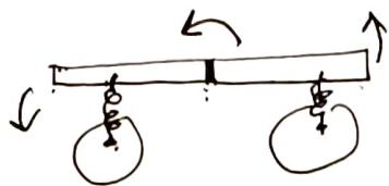
front and back leads to rotation of the angle of the body from the horizontal.
