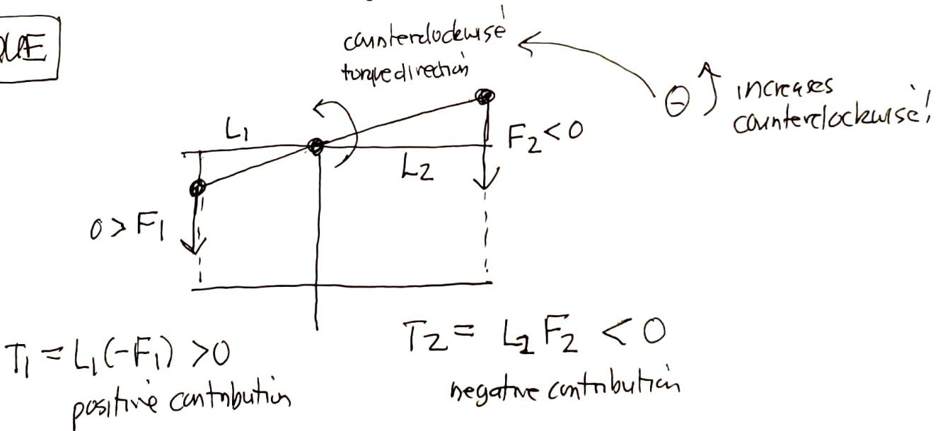
net counter-clockwise torque:
