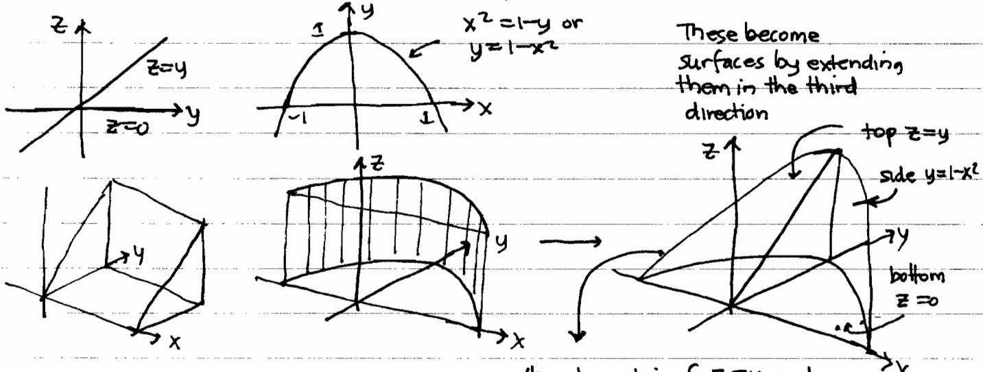
We now see the projections of this solid onto the 3 coordinate planes, each of which corresponds to the region of the outer double integral which can be iterated in two ways, while the inner integral is in the third coordinate which has to be given a starting and stopping value
