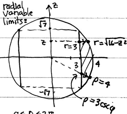
3 in radius hole in 4 in radius sphere
