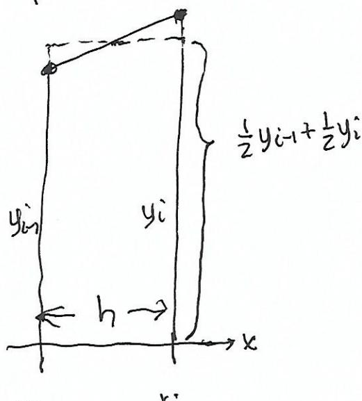
$$\Delta A_i = \underbrace{h}_{\text{width}} \underbrace{\left( \frac{1}{2}y_{i-1} + \frac{1}{2}y_i \right)}_{\text{height of equivalent rectangle}}$$
